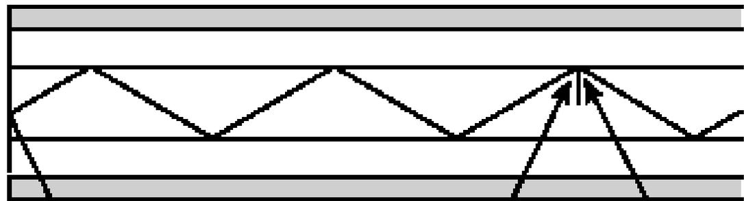
Light at less than critical angle is absorbed in jacket
