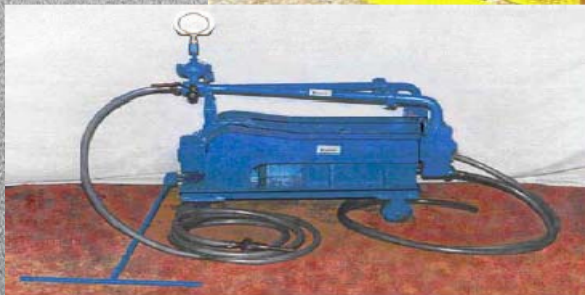
Gambar 2.44 Pompa Grouting Model 3-600 Produksi Fressynet
