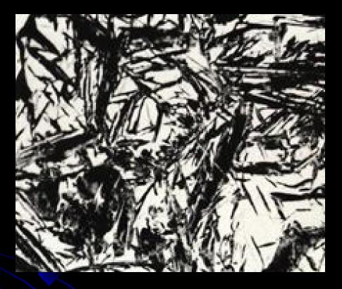
The needle-like structure of martensite, the white areas are retained austenite.
