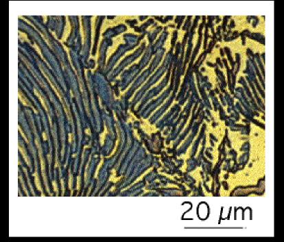
Two-dimensional view of pearlite, consisting of alternating layers of cementite and ferrite.
